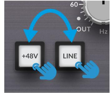
In this mode it's also possible to test the correct operation of the potentiometers. A position change on any of the pots will trigger the relay to click as a confirmation feedback.
