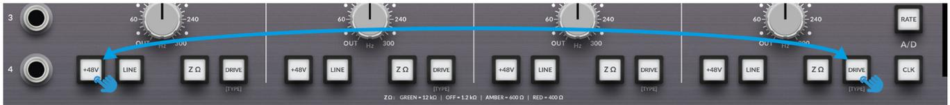
*Press and hold both Channel 1 +48V and Channel 4 DRIVE buttons during boot to trigger a factory reset.*
