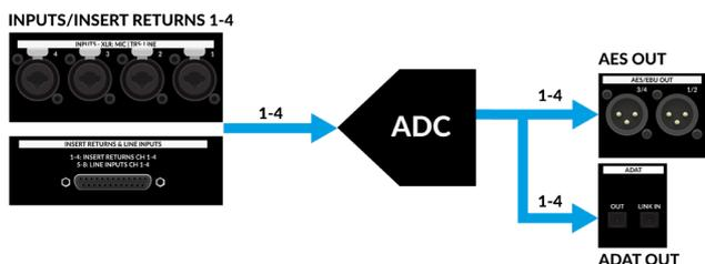
Normal mode - AES and ADAT Outputs fed from A-D converter
