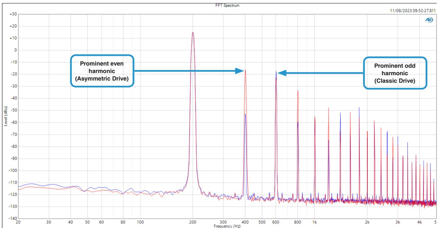
*Test tone 200 Hz, 29 dB Gain, input level -14.35 dBu.*
