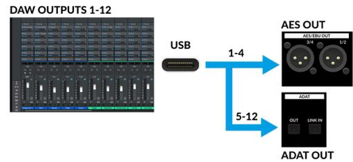
DAW feeds digital outputs mode - AES and ADAT fed from USB. Example given at 44.1/48 kHz
